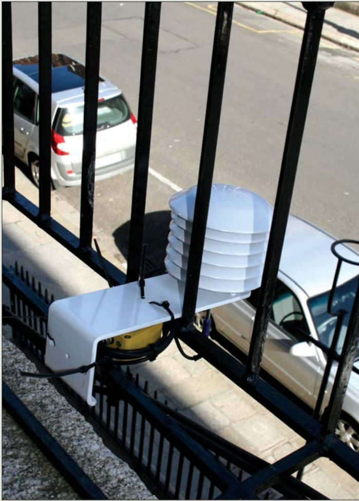
(left) a wireless external air temperature monitor
